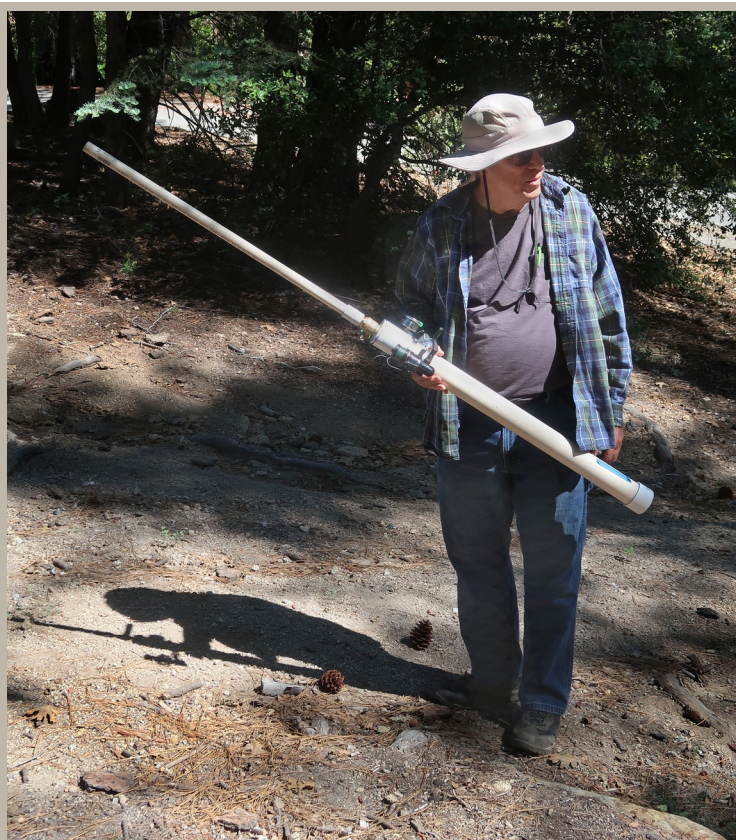
Larry AD6G with his DIY air launcher, “a device to pneumatically launch a fishing line into the air and over a tree.” – Photo by Lis Schwitters N6NDC
