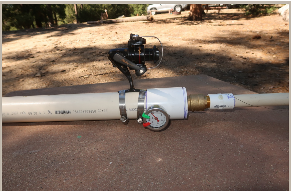
A closer view of the "air launcher". – Photo by Lis Schwitters N6NDC
