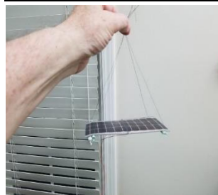
Shown is the finished tracker we are flying for W5KUB-18. The tracker and voltage regulator are glued and taped under the back side of the solar panel. The gps antenna sticks up off the edge of the panel. A 20 meter dipole completes the entire system.
