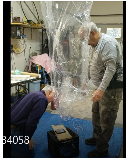
Ed and Tom precisely filling the sbs-13 balloon with 8 grams of free lift.
