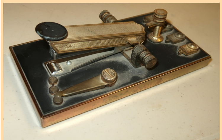
A key made from a stapler was among the presented items from Bill's station. – Photo by Lis N6NDC
