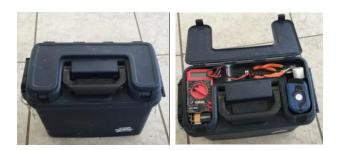
In the very bottom, just visible are the 2 10 Ah gell cells, each individually fused. On the right hand side the 12v to 110v 400 watt converter. The Power Poles on the lid, allow a vehicle to be connected, so I can use its battery in the vehicle, or if the engine is running, charge these batteries. On the floor is the 12v SLA battery charger (home built using a UC3906N, schematic available on request). In the cardboard tube are 2 110v LED lights, a homemade 12v LED light is in the bottom.
