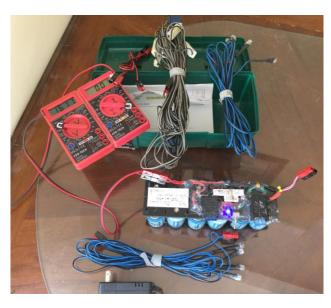
A close up of some of the 10000mAh cells. A slight problem with this set up is the running voltage of the pack is 16 volts average. A little high for most radios, but I have included a couple of resistors on top to limit the current, so as to be able to somewhat part charge a 12 volt battery, and to charge some of the cells from a 12v car battery. The switch changes the output voltage from 16v to 4.8v. Schematic on request.
