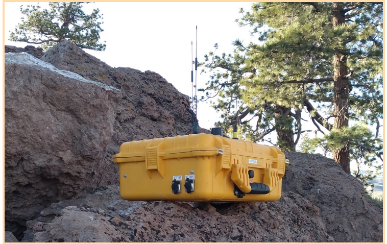
"Chris WB6CDF 's portable WiFi/Verizon Internet [router]. Used to link our logging software." – Larry AD6G
