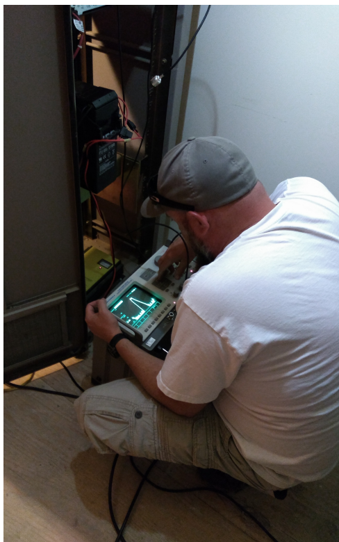
Chris WB6CDF checks the duplexer using a communications analyzer. — Photo by AD6G
